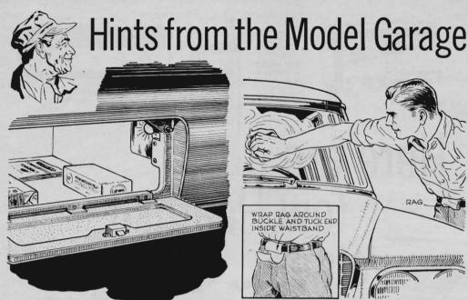
You'll have more light in your glove box if you line the inside of the compartment with white polyurethane foam plastic and glue a small mirror behind the bulb. The foam lining also will reduce rattling of loose objects and help prevent breakage.
