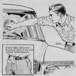
To prevent scratching fenders with belt buckles when leaning over to clean windshields, service-station men may want to try this hint: Wrap a small rag or handkerchief around the buckle; tuck the loose end inside the waistband so it won't slip.
