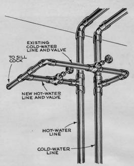
When washing your car in wintertime, the water can get numbingly cold if your garage has only a cold-water line. By connecting a hot-water line from the basement you can have warm water. A shutoff valve lets you turn off hot water in the summer.
