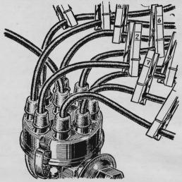
To keep from mixing up spark-plug leads, clip a numbered clothespin to each lead before removing it. Also, mark the numberone terminal on the distributor. With leads numbered according to firing order, it's an easy job to replace them properly.
