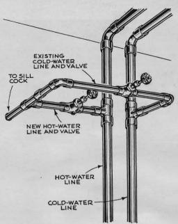
When washing your car in wintertime, the water can get numbingly cold if your garage has only a cold-water line. By connecting a hot-water line from the basement you can have warm water. A shutoff valve lets you turn off hot water in the summer.
