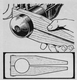
Can't unscrew your oil filter by hand? Make a wrench from two pieces of 3" board, each 16" by 2½". Cut a hole between the two halves %" smaller than the diameter of the filter. Attach halves with four nails and a strip from a tin can.
