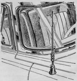
A broken aerial needn't be replaced. Fix it with a compression coupling of the type used to join copper lines. You'll get a permanent repair without soldering or flaring the aerial ends. The %" connector is just right for most aerials.
