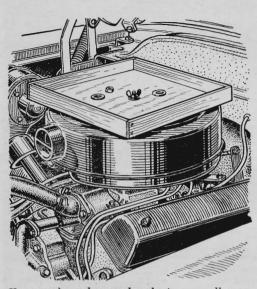
Keep tools and parts handy in a small tray made of wood scraps when you work under the hood. Drill a hole in the center to accept the air-cleaner bolt; fasten with the original wingnut. This works fine—except when the carb needs attention.
