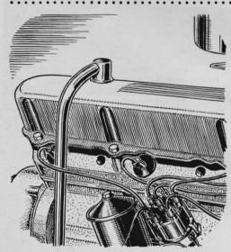
An engine that wouldn't crank fast enough to start because of cold—this was one reader's problem. He removed every other spark plug to gain cranking speed. The engine started, soon warmed up. He shut it off, replaced the plugs, restarted easily.
