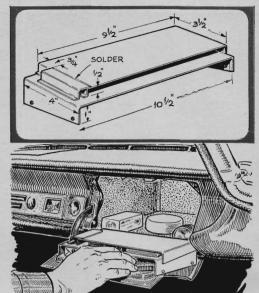
To keep your glove box neat, make this dual-compartment container from sheet copper and mount it on the inside of the lid. Roll the front edges for safety. The dimensions given are for 1958-62 Ramblers, but they can be changed to fit other cars.
