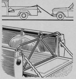
You can improve traction of a two-wheel-drive tow truck with a welded tubular framework that raises the tow line at the rear. This also allows the truck springs to cushion the pull. Weld a ring to the top of the frame to guide the tow line.
