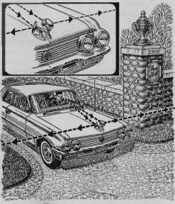
To see into blind intersections without pulling out dangerously far, try these two small hood-mounted mirrors. Most mirrors have a limited range of adjustment, so toe them in 25 degrees. On bare late-model hoods, the mirrors double as ornaments.
