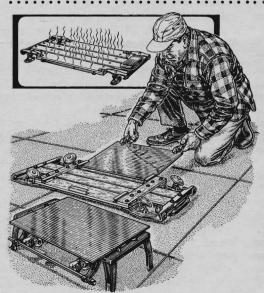
A warm creeper is welcome on a cold day when you make repairs outdoors. Heat a piece of 18"-by-30" boiler plate on a garage stove; it'll stay hot several minutes. U brackets hold it under the creeper. Keep a second plate heating on the stove.
