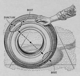
When repairing a tire casing with a boot, install a second boot of the same size directly opposite the first. This helps balance the wheel. The cost of the extra boot is well worth while, since vibration and wheel tramp at speed are eliminated.
