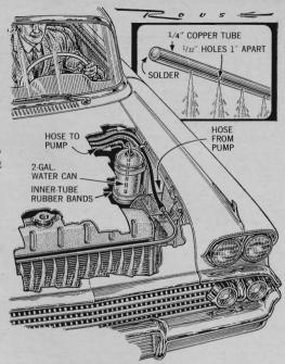
When towing a trailer in mountain country one reader prevented overheating by running a hose from the windshield-washer pump to a copper tube over the radiator. Water from a two-gallon can squirts from holes drilled in the tube, providing cooling.
