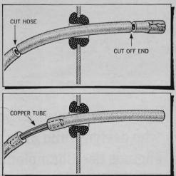
A cracked end on a vacuum hose doesn't necessarily mean replacement of the entire hose. Cut the hose in half under the hood and insert a piece of copper tubing for added length. Snip off the worn end and replace the hose on the fitting.
