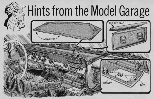
Small magnets make good fasteners for many auto accessories. Sew several into the hem of a dark-colored cloth and apply it to your dashboard top to prevent glare. Or cement two magnets to the back of a sunglasses case. This keeps the glasses on the dashboard, where they're handy. Cutting off the flap makes it easier to remove the glasses. An envelope taped to the glovebox lid holds credit-card receipts and trading stamps neatly; a magnet cemented to the flap keeps the envelope closed.
