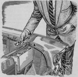
A permanently mounted toolbox under the hood keeps small tools, tire gauge, spare fuses, and dipstick rag handy. Use a two-quart metal container, cutting one side away and rolling under the sharp edges. Paint it and mount with existing bolts.
