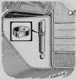
Keep flares within easy reach for any emergency. Mount them with spring-type hammer clamps (the kind used on workbench tool boards) on the kickpads ahead of the doors, using existing screws. Press a protective cork on a spike-bottomed fuse.
