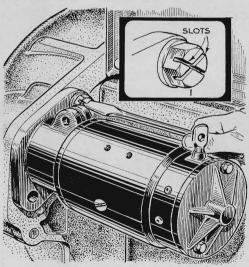
Hard-to-reach bolts like those on top of many starter motors can be engaged easily with a screwdriver if you cut an X-shaped notch in the head with a hacksaw. After the bolt has been screwed in, it can be tightened with an ordinary wrench.
