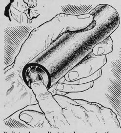
Radiator hoses slip into place easier if you smear the first inch or so of the hose on the inside with graphite jointing compound. Apply the stuff to the radiator or engine pipe, too. The compound also helps you get a good, tight seal at the joint.
