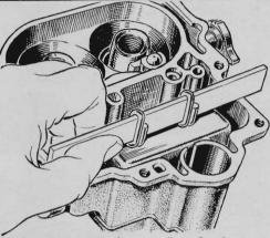
Make your own carburetor-float depth gauge with a straightedge about 6" long and two short lengths of wire with a diameter equal to the desired float depth. Wrap the two lengths of wire snugly several times around the straightedge about 14" apart.
