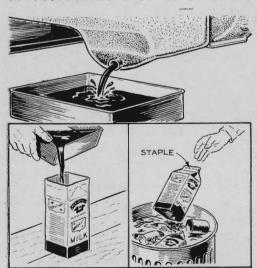
Getting rid of dirty engine oil needn't be a problem. Place a pan under the crankcase while draining it. Then pour the oil into an empty milk carton, staple the top shut, and toss the carton into the garbage can. The waxed container won't leak.
