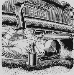
A flashlight makes a good trouble light when you're making repairs under a car. To one corner of your creeper attach a tin can with its top removed. Put the flashlight in the can. It's easy to aim the light anywhere you need it.
