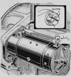
Hard-to-reach bolts like those on top of many starter motors can be engaged easily with a screwdriver if you cut an X-shaped notch in the head with a hacksaw. After the bolt has been screwed in, it can be tightened with an ordinary wrench.
