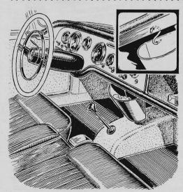
Mount a litter basket with a metal showercurtain hook, using one of the many accessory holes that are factory-drilled at the bottom of the dashboard cowling. Hang the basket right over the transmission hump to keep it from taking up passenger leg room.
