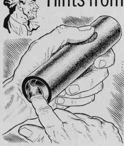
Radiator hoses slip into place easier if you smear the first inch or so of the hose on the inside with graphite jointing compound. Apply the stuff to the radiator or engine pipe, too. The compound also helps you get a good, tight seal at the joint.
