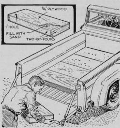
Need ballast in your pickup truck when it snows? Five of these sandboxes take up little space, and they won't slide around. Tops and bottoms are %-inch plywood; sides are two-by-fours. A one-inch hole in the top of one lets you use sand on ice.
