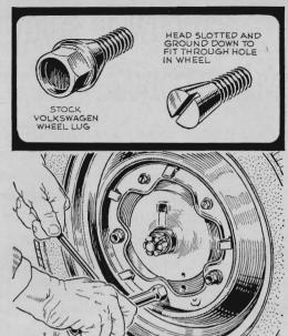
VW brake drums have no studs for positioning a wheel when changing tires. You can make temporary ones by grinding down two extra wheel lugs. Saw screwdriver slots. Before removing wheel, temporarily replace two lugs with the screw-in studs.
