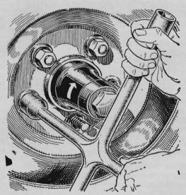
Small arrows painted on axle hubs will remind you to turn the lug bolts in the proper direction when you're changing a tire. This is particularly handy on cars that have a left-hand thread on one side and a right-hand thread on the other.
