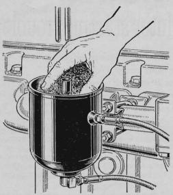
Cleaning sludge from an oil filter is easy with highly absorbent lint salvaged from a clothes dryer. Wad the lint into a ball and push it down into the filter. When the oil is soaked up, wipe the inside of the filter clean with a lint-free rag.
