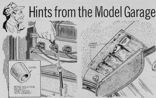
A cork stopper speeds up oil checks on engines in which the dipstick tube is hard to see. Instead of groping or using a flashlight, paint the stopper white, drill a hole through it, and cement it in place over the end of the dipstick tube.
