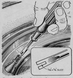
Removing the valve stem from a tire is an easy job with this homemade valve tool. Cut a 1/4" slot in the tip of a thin-bladed screwdriver with a hacksaw and file. You may have to grind down the edges of the blade so it will fit inside the valve.
