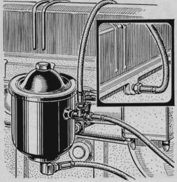
Fouled rocker-arm oil lines are common on certain sixes. Easy fix: Install a tee fitting on the oil-filter outlet. Then run a flex line from the tee to the clean-out hole on the right side of the block to feed oil directly from the filter to the rocker arms.
