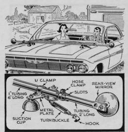
Extend these mirrors when towing a trailer and push them in when the trailer is unhitched. Accessory mirrors are attached to 2' aluminum tubes that telescope into a 6'-long, 1"-diameter tube with slotted ends. Clamps hold the extensions tight.
