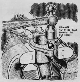
In making a gasket, you can locate and cut bolt holes in one step with a steel ball slightly larger than the hole. Shape the gasket and place it on one surface to be joined. Tap the ball lightly over the hole.
