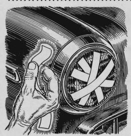
A strip of reflective tape, carried in the glove compartment, will protect you against collision if you're caught with a dead headlight. Strips pasted across the lens will show other motorists which light is out.
