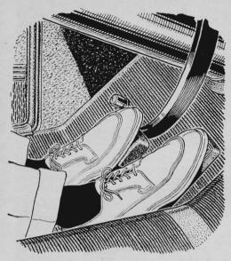
Keep brakes dry when driving through large puddles by lightly touching the brake pedal with your left foot and stepping on the gas with your right. This will hold brake linings against the drums, keeping water out and preventing fade or grabbing.
