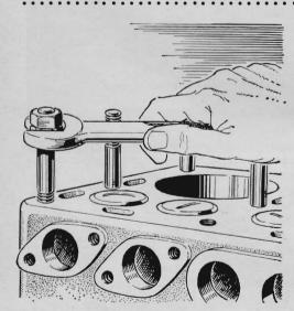
To remove a stud without stripping the thread, screw on a pair of nuts. Using two wrenches, jam the bottom nut against the top one. Additional pressure on the bottom nut will unscrew the stud. It's a simple matter to remove the nuts afterward.
