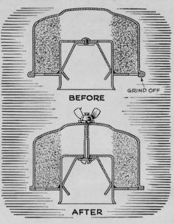
It's easier to clean the oil-breather cap on some cars if you grind away the rolled edge, drill a hole through the top of the cap, and insert a long bolt, lock washer, and wingnut. A dirty filter can be replaced with ordinary stainless-steel wool.
