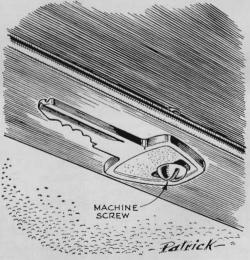
You won't get locked out of your car if you have a spare key. Find a spot to hide the key—under the gas-cap shield, under the hood, inside a fender—and drill and tap a hole. Attach the key with a machine screw. Use a dime to unscrew the key when needed.
