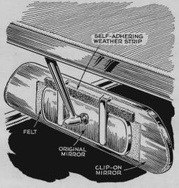
That oversize clip-on mirror won't loosen and rattle if mounted this way. Place a length of weather stripping just above the stock mirror to carry the weight of the clip-on. Cement a piece of felt to the back of the clip-on to absorb vibration.
