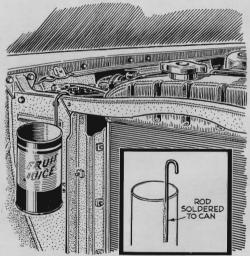
A container for holding small parts can be a big help when you're working under the hood. Use a small tin can and a foot-long piece of rod bent into the shape of a cane. Solder the rod to the can and form the hook to fit the top of the radiator guard.
