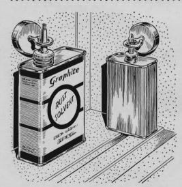
Hold cans upright in a truck bed with inexpensive, readily available magnetic cup hooks. Bend each hook closed to form an eye. When slipped over the neck of the can, the eye keeps the can from overturning and perhaps spilling its contents.
