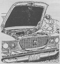
When adjusting the cark on an alternatorequipped car, turn on the lights. If you don't, idle speed will be too low at night when lights are used. Alternators have a higher output at idle than generators, but they also drain more engine power.
