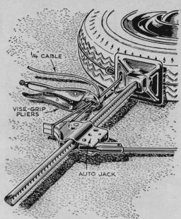
To inflate a tubeless tire, you need a good seal between bead and rim. Try running a cable lasso around the crown, passing the free end through the base hole of your jack and around the lift finger. Work jack to compress the tire till it holds air.
