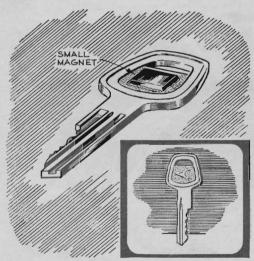
You'll never be locked out if you hide a spare door key where its accessible from the outside. A simple way to attach it to the car body is to fasten a small magnet to the head with epoxy glue. The type of magnet often sewn on potholders is ideal.
