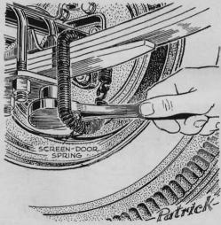
When removing U bolts from auto springs, keep a socket wrench seated on the nut by looping a screen-door spring around the axle or spring. Slip wrench through the sling, which should be snug enough to exert tension. Wrench can be turned with one hand.
