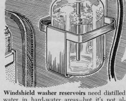
Windshield washer reservoirs need distilled water in hard-water areas—but it's not always easy to come by. For a substitute, collect water from melting ice when you defrost your refrigerator or from the plastic drain pan of an electric dehumidifier.
