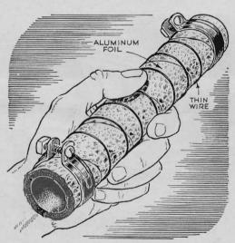
Radiator and heater hoses are too often located near oil dipstick tubes and valve covers, where they get coated with oil and start to deteriorate. To prevent this, give such hoses a jacket of foil, held in place with a wrapping of light wire.
