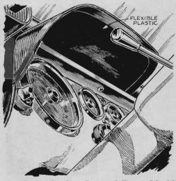
A plastic "eyebrow" can kill windshield reflections from a lighted instrument panel. Cut it from flexible opaque sheet, loosen the molding enough to slip the edge under, then retighten. If dash lacks molding, drift holes for sheet-metal screws.
