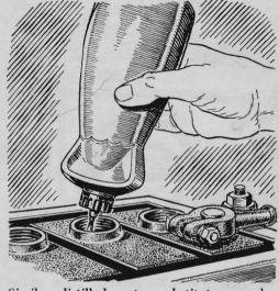
Similar distilled water substitutes can be used in your battery. You can carry a ready supply in your car by filling a plastic detergent bottle. Drill a 1/16" hole in the cap tip from the inside, and clean the bottle thoroughly before you fill it.
