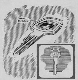
You'll never be locked out if you hide a spare door key where its accessible from the outside. A simple way to attach it to the car body is to fasten a small magnet to the head with epoxy glue. The type of magnet often sewn on potholders is ideal.
