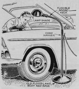
Put light where it's needed, when you're working under the hood or inside the body of a car, by rigging up this light stand. Connect a gooseneck desk lamp to an old floor-lamp stand. Add a hook to store the coiled cord when the lamp's not in use.
