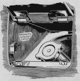
oil. By cementing a small magnet to the plug, you can keep it beside the drain hole. Or, if the gas-tank lid fails to close, buy a magnetic door catch. Drill two holes inside the gas well, then attach the catch so the lid touches the magnet in the closed position.
