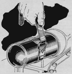
Changing a throw-away oil filter can mean a lot of struggling. Try using an old leather strap and buckle to remove it. Just slip the looped belt over the filter, tighten it up, and lift it out. The tightened strap will keep it from slipping.
