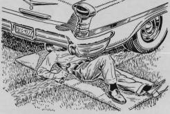
A slippery folding plastic mat allows you to slide easily under a car to make repairs. Make it of a 36"-by-72" sheet of roll plastic and four large newspapers. Fold the plastic lengthwise over the papers. Sew around the borders and between the papers.
