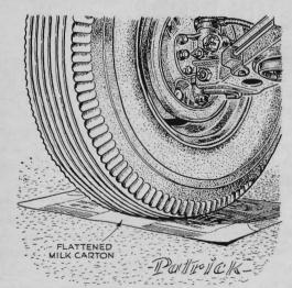
Reaching ball joints with a grease gun requires moving the front wheels. This is easier if the wheels rest on a slippery surface. Cut the ends off two milk cartons, flatten them, and put them under the tires. It also saves wear on the steering linkage.
