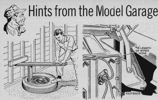
Stubborn tire beads can be broken loose easily with this setup. Place a two-by-four under a brace or car bumper. The fulcrum, on the tire, should be slightly higher than the brace. Use a lever long enough to provide good mechanical advantage.
