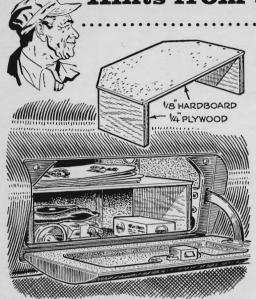
A glove-compartment shelf lets you make better use of limited space by filing road maps up out of the way. It's easily made of  $\frac{1}{8}$ " hardboard with  $\frac{1}{4}$ " plywood for the supports. Make a cardboard pattern first to insure proper fit.
