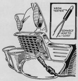
other tip for engine-block heaters: To make sure the heater is working, hook up a neon-tube tester. Run the leads inside the heater-cord plug and tape the tester to the cord, covering all but the light. If the tester lights, you have current.
