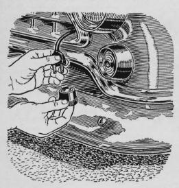
Engine-block heater plugs stay clean if protected by an electric-cord connector. The heater warms the water in the cooling system—a big help in cold climes—but efficiency is reduced when plug prongs are corroded by air or water. An-
