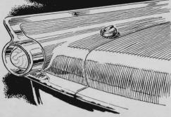
Collar your gas cap with a strip of foam rubber, cork, or felt glued in place. It will keep the car paint from being scratched by pumpmen who plunk the cap on a fender or deck lid. Extend the strip % inch below the cap's base to act as a cushion.
