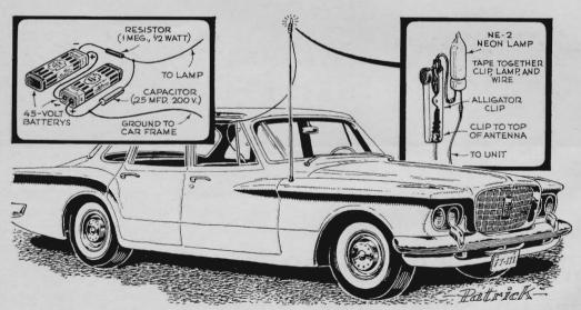
Finding your car at night, particularly in a big parking lot, can be a problem. But this tiny antenna light will guide you to it every time. You'll need two 45-volt batteries, a resistor, a capacitor, and a length of small-gauge insulated wire running to a neon bulb
