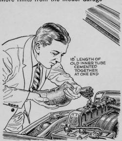
If your radiator boils over, an 18-inch section of old inner tube cemented closed at one end makes a handy refiller. Use it to carry water to your car from a nearby stream or tap. When not in use, the flexible bucket rolls up for compact storage.
