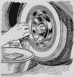
Whitewalls come out whiter than new when cleaned with a small wire brush and powdered household cleanser containing bleach. Wet the tires before scrubbing them. To prevent damage to the rubber, carefully rinse off all the cleanser afterward.
