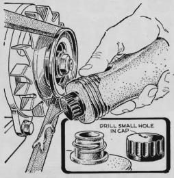
Squirting belt dressing or oil into hard-toreach spots is easy with a plastic liquid-detergent container. Drill a small hole in the cap, and fill the container with oil or any other liquid you want to spray. To squirt, just squeeze the sides of the bottle.
