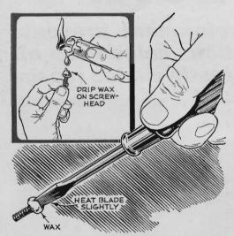
Starting a screw by hand is difficult if it's behind a dashboard or in other confined areas. Here's one way to make the screw stick to the screwdriver blade: Drip candle wax on the screwhead, heat the blade slightly, and press it into the screw slot.
