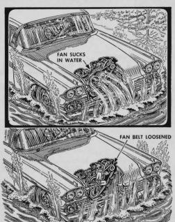
Engines often wet out when driven through a flooded roadway. The radiator fan usually is the culprit; it sucks up the water and throws it back onto ignition wiring. Next time, loosen the fan belt so the fan doesn't turn. Reconnect it on dry ground.
