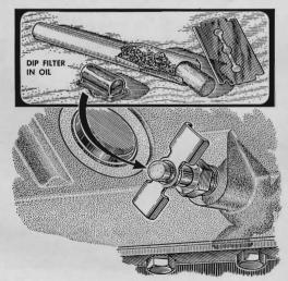
Dirt won't clog petcocks on radiator and engine block if you insert cigarette filters that have been soaked in oil. Leave ¼" protruding. The filters also prevent messy dripping and keep hands dry while you're opening the petcocks to drain the water.
