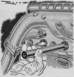
You can remove hot spark plugs without burning your hands by means of a piece of garden hose. Loosen the plugs with a wrench, slip on an 8" section of hose, and unscrew them. If plugs are small, slip hose over base and bear down while turning.
