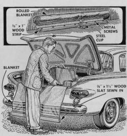
An old blanket can keep you clean when you unload your car trunk. It protects clothing from grime on the bumper. Fasten the blanket to the trunk floor, and sew a wooden slat into the edge to prevent flapping. The blanket rolls up when not in use.
