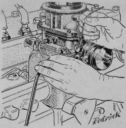
Trouble with an automatic choxe? If the manifold tube is clogged, you may be able to clear it by alternately squirting in penetrating oil and inserting a steel wire an inch or two at a time. When oil drains out the bottom, reconnect the tube.
