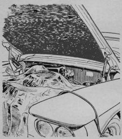
Nestle a trouble light next to the carburetor for quick starts on cold mornings. To keep the heat from dissipating too quickly to do any good, blanket the radiator and engine with a sheet of plastic film of the type used for storm windows.
