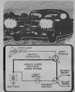
Control a spotlight automatically by wiring a single-pole, double-throw toggle switch into the line. With toggle in A (automatic) position, the spot goes off when you change to low beam. For normal operation, flip toggle to N position.
