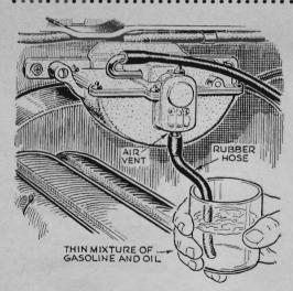
A windshield-wiper motor can sometimes be serviced without disassembly. If the piston flap has dried out and doesn't seal, try lubricating it as shown. With wipers operating, the vacuum draws the gas-oil mainture into the dry chamber.
