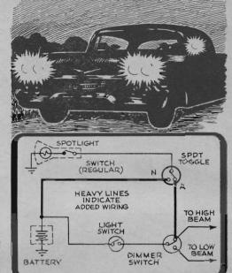
Control a spotlight automatically by wiring a single-pole, double-throw toggle switch into the line. With toggle in A (automatic) position, the spot goes off when you change to low beam. For normal operation, flip toggle to N position.
