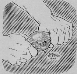
**Greasing a wheel bearing** needn't be a messy or tedious job. Merely place the bearing and a generous supply of grease in a small plastic bag, grasp each end, and squeeze the grease around the bearing, manipulating with your fingers.
