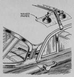
Roof marks left by rubber bases of cartop carriers are often hard to remove from light-colored cars. To avoid this chore after each short-distance haul, one motorist slips waxed paper under the cups before cinching the strap.
