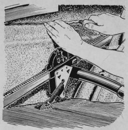
To anchor loose wiring under the hood and dashboard, or in the trunk, squeeze a bead of hard-setting sealant (such as Permatex Form-A-Gasket #1) along the wire's proper path and press the wire in place. It can be pulled loose any time.
