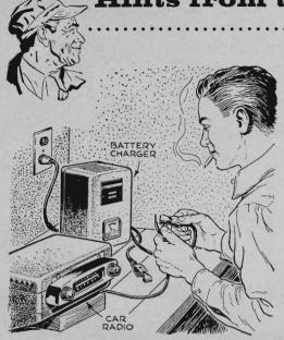
**Trouble-shooting a radio** or other electrical accessory from your car requires a low-voltage power source. A battery charger plugged into the house current acts as a converter. Just be sure its output is more than the accessory consumes.
