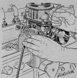
Trouble with an automatic choke? If the manifold tube is clogged, you may be able to clear it by alternately squirting in penetrating oil and inserting a steel wire an inch or two at a time. When oil drains out the bottom, reconnect the tube.
