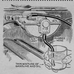
A windshield-wiper motor can sometimes be serviced without disassembly. If the piston flap has dried out and doesn't seal, try lubricating it as shown. With wipers operating, the vacuum draws the gas-oil naixture into the dry chamber.
