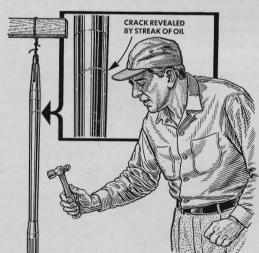
An invisible crack in a rear-axle shaft can be detected without fancy equipment. Clean the shaft with solvent, wipe dry, and hang it up with wire. Then tap with a hammer to expel solvent and oil—and pinpoint the crack.
