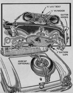
This deck-top spare-tire holder is ideal when every bit of trunk space is needed for vacation luggage. Double web straps pass through wheel slits, securing the wheel. Plywood backing plate has three big suction cups so finish isn't marred.
