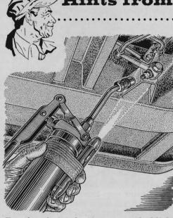
For chassis lubrication, a pen flashlight securely taped to the barrel of a grease gun is handier than an extension trouble light. Just locate each grease fitting with the concentrated beam of light and you're automatically on the target.
