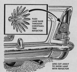
**Stop lights glow brighter** with the help of Christmas-tree reflectors. Slip the base of the bulb through the reflector and mount it in the light socket. The reflector may have to be trimmed to fit inside some of the smaller tail lenses.
