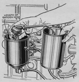
Changing an oil-filter cartridge gets messy when it's time to drain dirty oil from the filter case. A neat way: Pump out the oil with a plunger from an oil squirt can connected to a piece of old garden hose. Tape the plunger shaft for a good seal.
