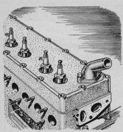
To free a cylinder head that's "frozen" to the block, try this easy trick: After you have removed all retaining nuts and bolts, engage the starter. This will build up sufficient compression to loosen and lift the head and save you a struggle.
