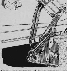
Check the position of hood springs before you unfasten them to remove the hood for major engine work. Reversing the direction of the spring hooks may prevent the hood from lining up properly with the cowl and fenders when you remount it.
