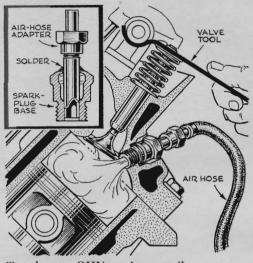
To change OHV springs easily, one mechanic does this: He screws an air hose into the spark-plug hole, using an old spark-plug base as an adapter. The valve is kept from moving into the cylinder by 80-100 p.s.i. Unplug the oil pan, set piston at TDC.
