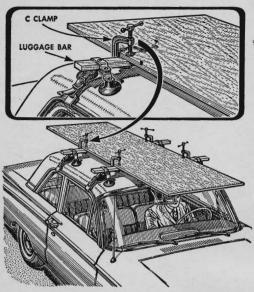
**C** clamps make car-top hauling easy, especially when you're carrying sheet materials such as plywood, fiberboard, or sheet rock. Clamping the cargo to the bars of the luggage carrier eliminates the need for securing with rope.
