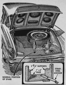
To increase luggage space, move your spare wheel from the trunk floor forward onto the shelf just behind the rear-seat cushion. Wood supports are easily cut with a jigsaw. No need to bolt down the wheel—it stays put even on rough roads.
