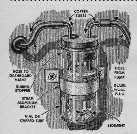
Windshield-washer clogging can be prevented with this homemade filter. Mounted in the water line between pump and dashboard valve, the four-inch vial or capped brass tube catches sediment. A glass-wool plug gives added filtration.
