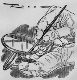
**Side-view mirrors last longer** if a thin line of clear lacquer is painted around the edge of the glass where it meets the metal. This keeps moisture from getting behind the glass and also helps prevent the mirror from loosening and rattling.
