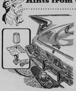
A trailer ball hitch won't rust while not in use if you place a few drops of heavy oil on it and cover it with a rag. Fold the rag to about four inches square. A wax-paper cup tied over the rag with strong cord gives extra protection.
