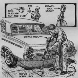
Fast jacking with a power impact tool. Remove handle from a tripod jack and replace it with the largest nut the impact tool will accept. Drill through nut and jackshaft, secure with pin, file pin flush. Engage the impact tool and let 'er go.
