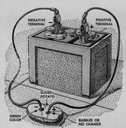
Which battery terminal is which? When corrosion obscures markings, half a potato can come to the rescue. Run leads from terminals into the potato, about an inch apart. Green color identifies negative lead. Positive lead may show bubbles.
