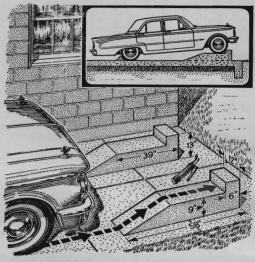
Two reinforced-concrete ramps built at any convenient spot will allow you to raise the front or rear of your car for home servicing and repairs. The car's track will determine ramp spacing. Use wheel chocks at opposite end for safety.
