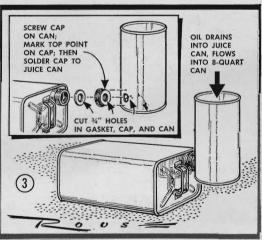
tered drips when removing the oil filter. (3) Solder a quart juice can to the cap of an eight-quart can and join them. The tall juice can will catch oil as it mans out of the crankcase. The oil will flow through the cap's hole to the large can.
