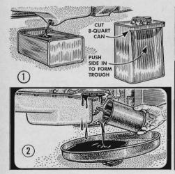
Tips on draining oil: (1) Slit an eightquart can near the top and press the side in. Oil will run down the trough and into the can, where it is retained when the can is picked up. (2) Use the lid from a garbage can to catch scat-
