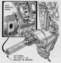
When making a hole in the dash or firewall, avoid the danger of drilling through into wiring or equipment by slipping a dowel over the drill bit to limit its penetration. Applying masking tape will keep the dowel end from chafing the finish.
