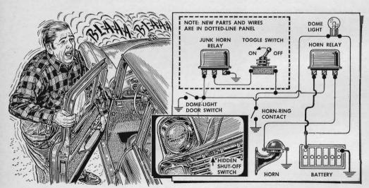
A thief will take off fast the moment he opens the door of a car equipped with this burglar alarm. The horn is the alarm, and it blows loudly and steadily when an intruder actuates the dome-light switch by opening the door. Slamming
