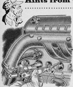
If a gasket sticks in the recess when you're removing spark plugs, fish it out safely and quickly with the hooked end of a wire-type gap gauge. Probing with the thin wire won't damage the threads or push dirt into the cylinder.
