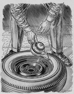
Air leaks at the rim seal of tubeless tires can be detected without immersing the wheel in a tank of water. Just lay the wheel flat, pour water around the rim, and watch for bubbles. Repeat the test on the other side of the wheel.
