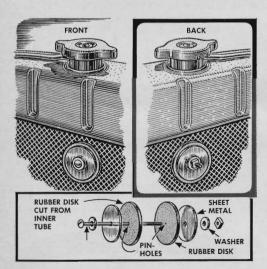
Radiator leaking? Expensive repairs can be postponed or avoided by sealing the ends of the core on both sides of the leak with disks cut from inner tube. Clamp the rubber in place with disks of metal, washers, and a long, thin bolt.
