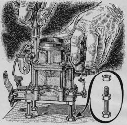
A steady work stand, made by locking four bolts in the holes at the base of a carburetor, will protect the linkage and throttle valves, and permit them to move freely while you're cleaning or overhauling the unit. Use two nuts on each bolt.
