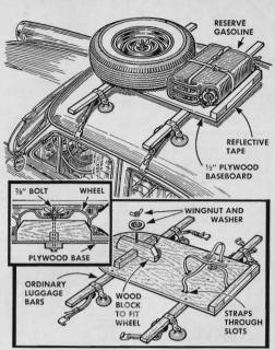
All the luggage around the spare tire will have to be unloaded if you have to change a flat on a trip. To avoid this, and to gain extra space for luggage, store the spare on top of the car, along with extra gas. Pack tools under a seat.
