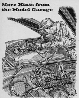
To keep a set of booster cables from becoming tangled when not in use, bind them together with electrician's tape at 12-inch intervals. Leave the ends free, so they can be separated far enough to reach the battery terminals.
