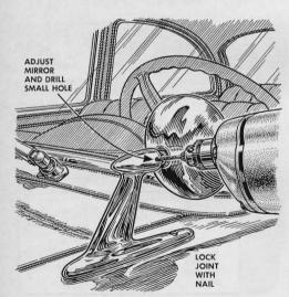
You can avoid the nuisance of readjusting the side-view mirror every time someone brushes against it by pinning it securely in position. Drill a small hole through the ball-and-socket joint and put a cotter pin or nail in the hole.
