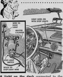
A light on the dash connected to the brake-light switch will indicate when stop lights go on. Knewing this, you can pump the pedal lightly to warn following drivers that you plan to stop before you apply full brake pressure.
