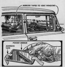
When towing a trailer or boat, you can command a full view of the rear on both sides by taping a small pocket mirror to the front vent windows. After determining the right height for the mirrors, adjust them by opening the windows.
