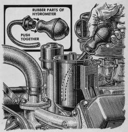
**Don't throw away** the rubber ends of a battery hydrometer if the glass tube breaks. Press the tip into the bulb and you'll have a syringe for adding water to the battery or drawing dirty oil from the bottom of the filter housing.
