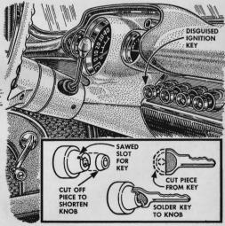
A car thief wouldn't think of starting your car by turning a knob on the dash. That's why you can leave this key in the ignition when making frequent stops. Get a matching knob and solder or cement the shank of a spare key to it.
