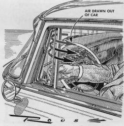
**Heater performance** can be greatly improved by opening the vent windows slightly. As air is drawn out of the car, a draft is created that increases the amount of fresh air that flows through the core of the heater.
