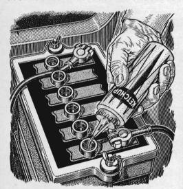
Want battery water handy in the garage? Instead of keeping it in a glass bottle, which will shatter if dropped or frozen, use a squeezable plastic ketchup dispenser. The thin spout meters water accurately, eliminating danger of overfilling.
