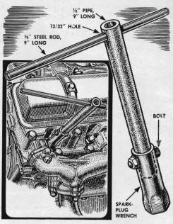
A short extension on your spark-plug wrench makes plug replacement easier and may save your wrist from being burned by a hot manifold. Drill holes at both ends of the pipe, one to bolt it to the wrench and the other for a T handle.
