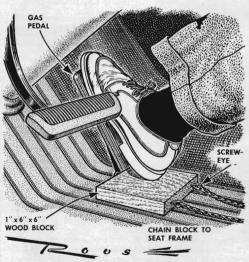
Change the angle of your foot on the gas pedal by resting the heel on a block of wood. It will make long trips less tiring. Chained to the seat frame, the block can't interfere with the brake and can be slid under the seat when not needed.
