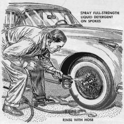
Cleaning wire wheels, usually a tedious job, can be speeded by spraying fullstrength detergent on them with an insect sprayer. Wait a few minutes for the detergent to work and flush with a garden hose hooked to a hot-water faucet.
