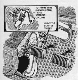
If a defective horn button on an older car or truck can't be fixed, substitute a foot switch. An old starter switch, mounted on the floorboard and wired to the horn, can be operated with your left foot. You may even like it better.
