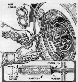
Make a speed wrench out of a lug wrench by cutting off the socket opposite the one you use for your car, and adding a wooden handle. Wrap the other two ends with solder to increase the flywheel effect when you spin the wrench.
