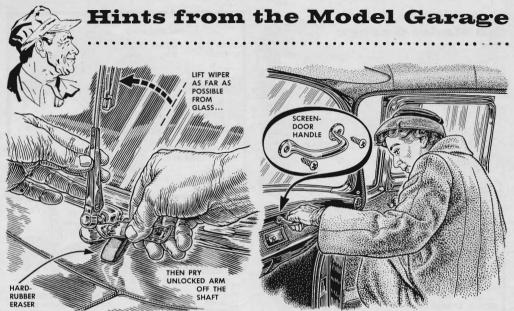
Remove a stuck wiper arm this way and you won't mar surrounding paint. Rest a beer-can opener on a hard-rubber eraser to give you a padded fulcrum and hook the point under the hub. The wiper arm can then be pried off easily.
