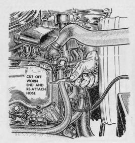
When installing a heater, leave some slack in the hose line. When the hose deteriorates at the engine—as it usually does first—you can cut off the bad end and reconnect the hose without installing a new line or draining the coolant.
