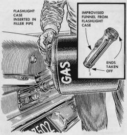
An emergency funnel for pouring gasoline from a can into a hard-to-reach filler pipe can be improvised from your car's flashlight. Remove both ends and the batteries, and insert the empty case into the filler pipe to extend it.
