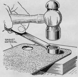
Holes can be punched in gasket material with a box wrench. Place the sheet on an anvil or other hard surface, hold the wrench in position, and tap it lightly with a hammer. To punch out a washer, use a small wrench followed by a larger.
