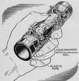
Radiator hoses—especially those at the bottom of the engine—deteriorate rapidly because of oil and dirt that accumulate on them. You can prolong their life by wrapping them with aluminum foil to keep them clean. Tape the ends of the foil.
