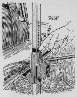
After taking off a flat tire, many motorists find they must jack up the car another inch or two in order to put on the spare. You can avoid this hazard by marking the proper height on the jack stand and raising the car to the mark.
