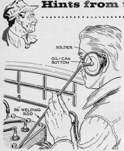
Want a homemade stethoscope that will help you track down engine noises? It's easy. Bend one end of a long rod and solder it to the bottom of an oil can. The can bottom acts as a diaphragm, amplifying the slightest sound.
