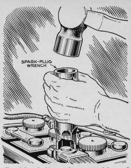
To drive battery clamps straight and securely onto terminal posts, place a spark-plug wrench on top and tap it gently. The hollow wrench end drives the clamps on without cocking or deforming them, as direct hammering often does.
