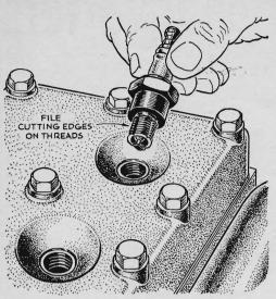
Clean engine threads when you're doing an overhaul by running dies on studs and taps into holes. An improvised tap for spark-plug holes can be made by filing notches across the threads on an old plug to give them a slight cutting edge.
