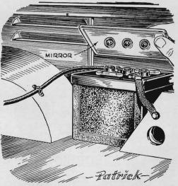
Check battery water with a mirror when you can't see easily into the cells, as in many foreign cars. It will save craning your neck and also eliminate the spillover of damaging acid that can occur if you attempt to fill a battery by guess.
