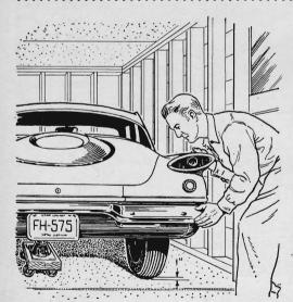
Need more work room in your garage? A car can be quickly shoved over this way to avoid repeated jockeying or in case the engine won't run. Place the jack on a wood block fitted with casters, raise the car 1" and push it sideways.
