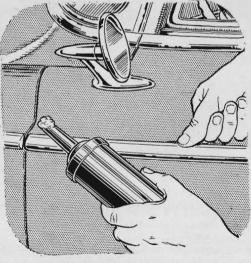
**Rust under molding strips** can be prevented by pressing calking compound between the *top* edge of each strip and the body of the car to keep slush and water from running in behind. Leave the bottom edge of the trim open for ventilation.
